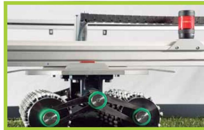
*We have one of the best in-house labs of the industry, with state-of-the-art equipment to test our turf during the design and quality control process. We use a Lisport machine (European Standard EN 15306) to simulate several years of heavy usage of our turf, to ensure we are producing products with dependable durability. We also use this machine to prepare “used” samples for our dealers, so customers can know exactly what to expect from the LikeGrass product line.*
