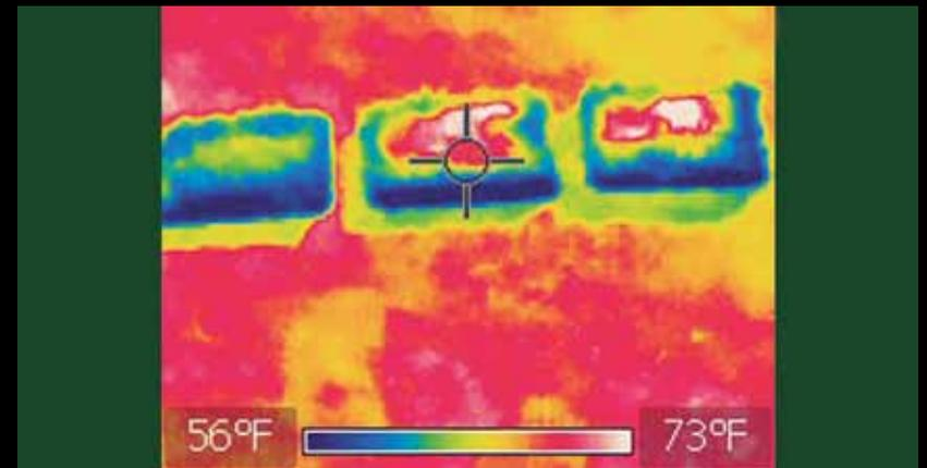
*This infrared image demonstrates that LikeGrass Reflective results in a cooler surface temperature. The image shows three turf samples placed on black asphalt, with an infill of 1 lb/sqf of black crumb rubber used with each sample. LikeGrass Reflective is on the left. The other two samples are standard 65 oz products. The blue color in the image is around 56° F; the white color is about 73° F.*
